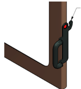
Illustration 8 – Lubrification du loquet
